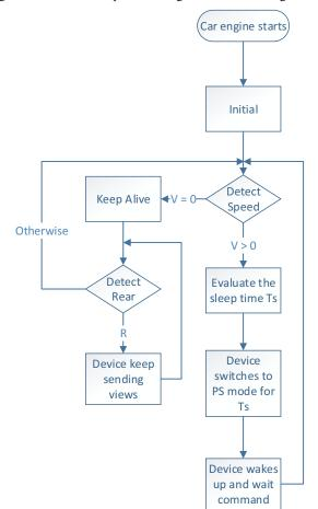
Fig. 4. Dynamic Power Saving Algorithm
