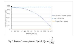
Fig 6 shows that the energy consumption of device is significantly deceased with rising speed. The reduced energy of device is shown in percentage as in TABLE III, when V is equal to zero, the reduced energy is 0.55%. When V speeds up to  $40 \, km \, dhr$ , the reduced energy is 7.61%. When V speeds up double than last, the reduce energy is coming to 34.83%. Finally, we can see that when the speed increase to 120km/hr, it realized highly energy efficient in Dynamic Power Saving.
