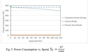
The comparison of three modes is shown in Fig 5, we suppose  $T_F = \frac{V^2}{1000}$  and find that the power consumption of device decreased a little with increasing speed. It verified that energy consumption can be reduced by the algorithm and shown in the TABLE II. The power consumption of device is proportional to speed.
